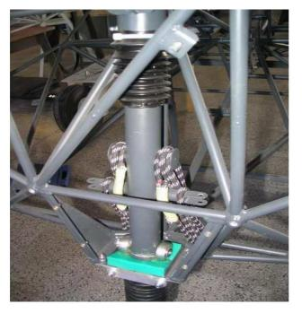
Fig.:Rubber cable suspension unit
