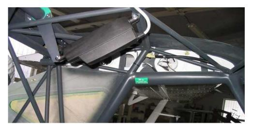
Fig.:Electric flap actuator
