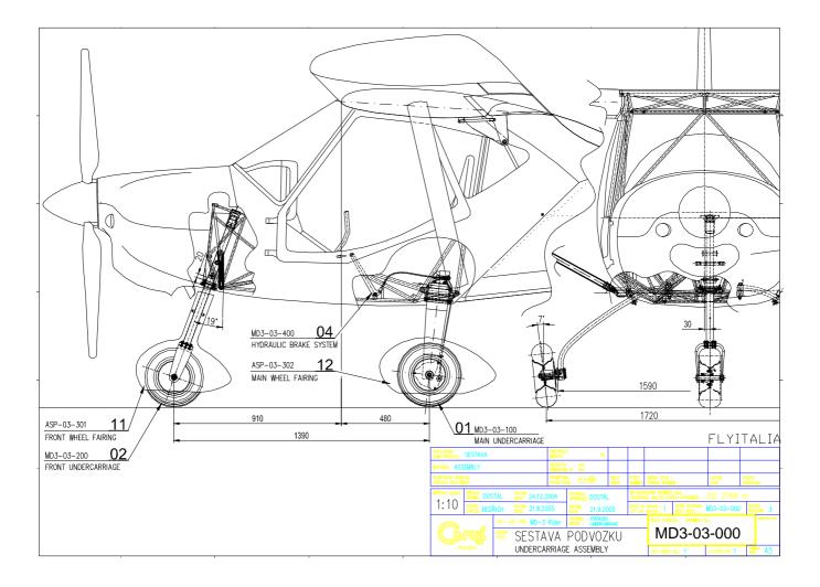
Fig.:Tricycle landing gear
