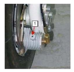
Fig.: Brake bleeding system 1. bleeding screw
