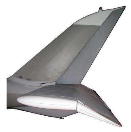
Classic-type all-metal TAIL has symmetrical NACA 12% profile. Horizontal Tail Unit (HTU) consists of stabilizer and elevator with trim tab. The semi monocoque construction consists of duralumin ribs, spars and skin. Construction is riveted by blind rivets and glued by Efimastic PU50.
