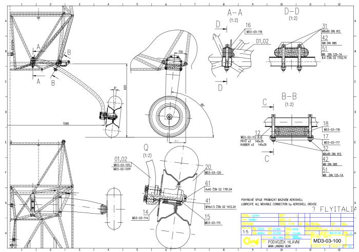
Fig.: Main landing gear
