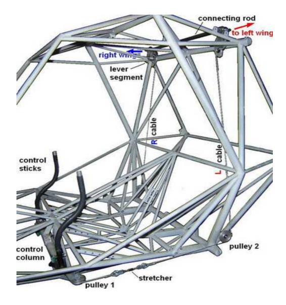
Fig.:Ailerons control system
