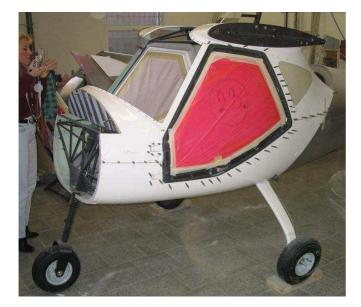
Cockpit fairing is produced from glass fiber composite, glued on the tubes and sheets of airframe and covers firewall, instrument panel including air vents, windshield frame in the front, conection to the wings in the top and door frames on the sides. In the rear COCKPIT FAIRING is equipped by foldable cargo compartment doors, needed to be folded for wing folding too.
