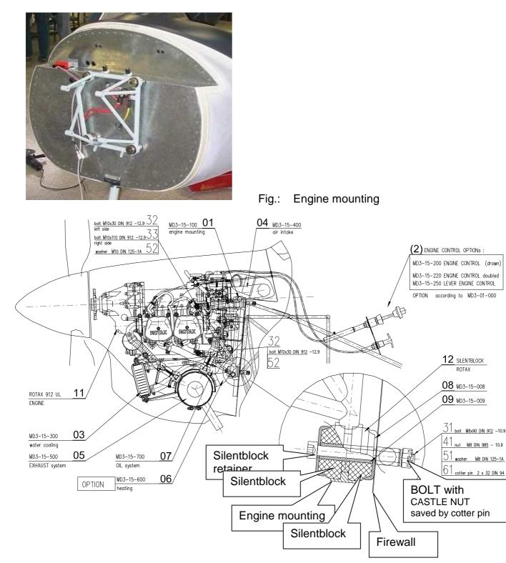
Fig.: Engine mounting suspensions
