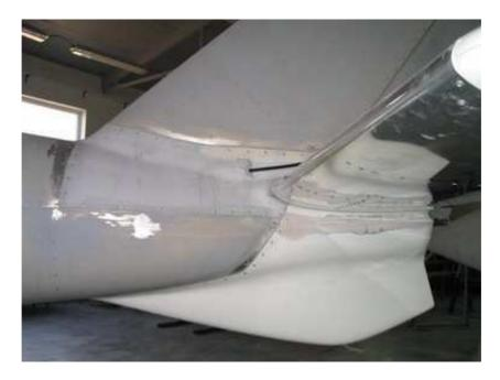
Fig.: Auxiliary tail skid
