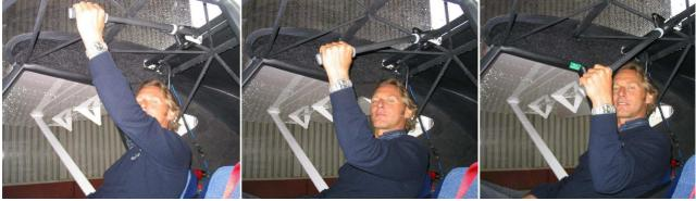
Basic UL version uses ceiling placed hand operated lever for flaps acuating
