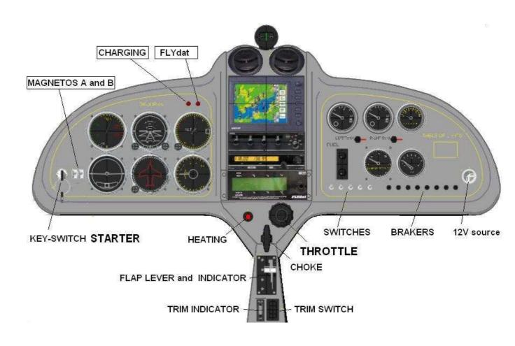
Fig.:Example of panel included standard analog instruments
