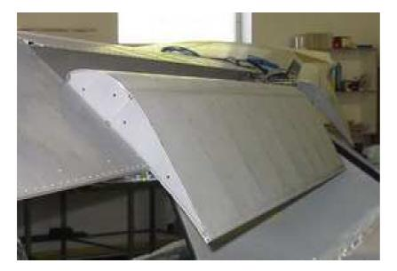
Fig.: Flaps in landing position
