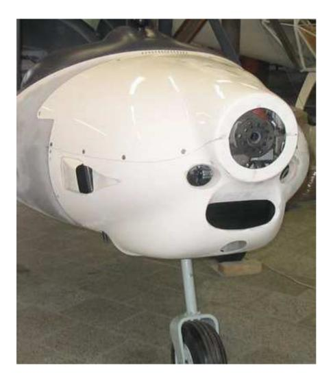
Fig.: Engine cowlings
